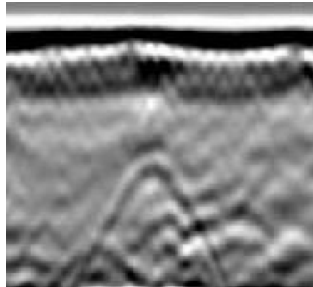
Fig. 2 Underground pipe reflection
